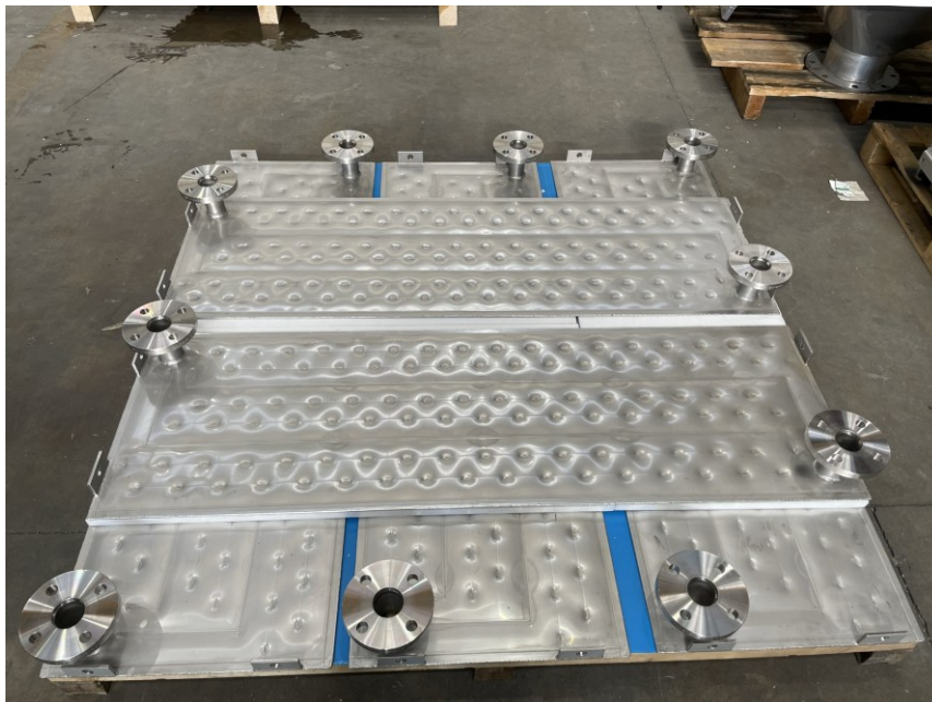
Figure 5.5: Stack of single embossed pillow plates before shipment. The designed application is for heating preexisting tanks, through application on lateral surfaces with heat transfer mastic.
