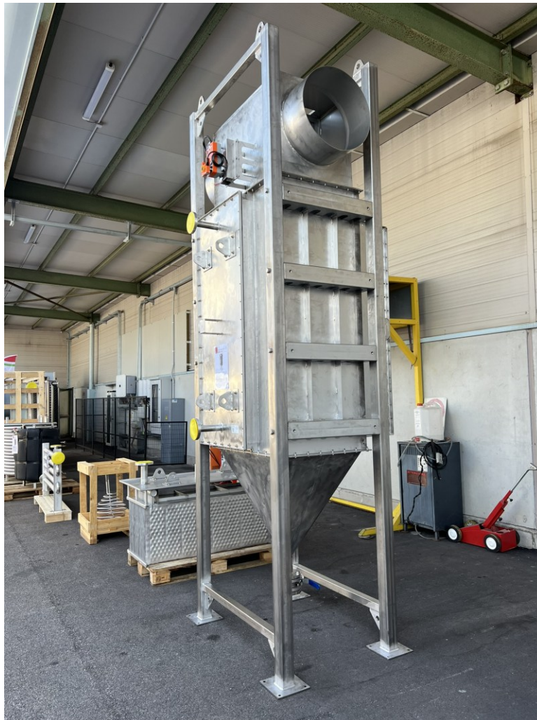
Figure 5.10: PPHE for heat recovery from biomass smoke, featuring an extractable PPHE cartridge, motorized bypass, soot collection at the bottom and bolt on frame for easy transport and final positioning
