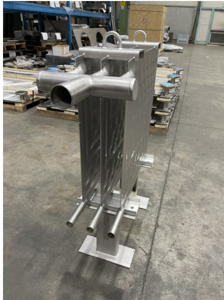
Figure 5.4: A steam powered PPHE for natural convection heating of a tank. Modular prototype which originated two recorded productions.
