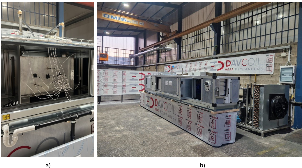
Figure 3.9: Pictures of the Condensation Heat Recovery experimental set-up, with a particular of the PPHE during sensor installation (a), and the entire system after the initial positioning (b).
