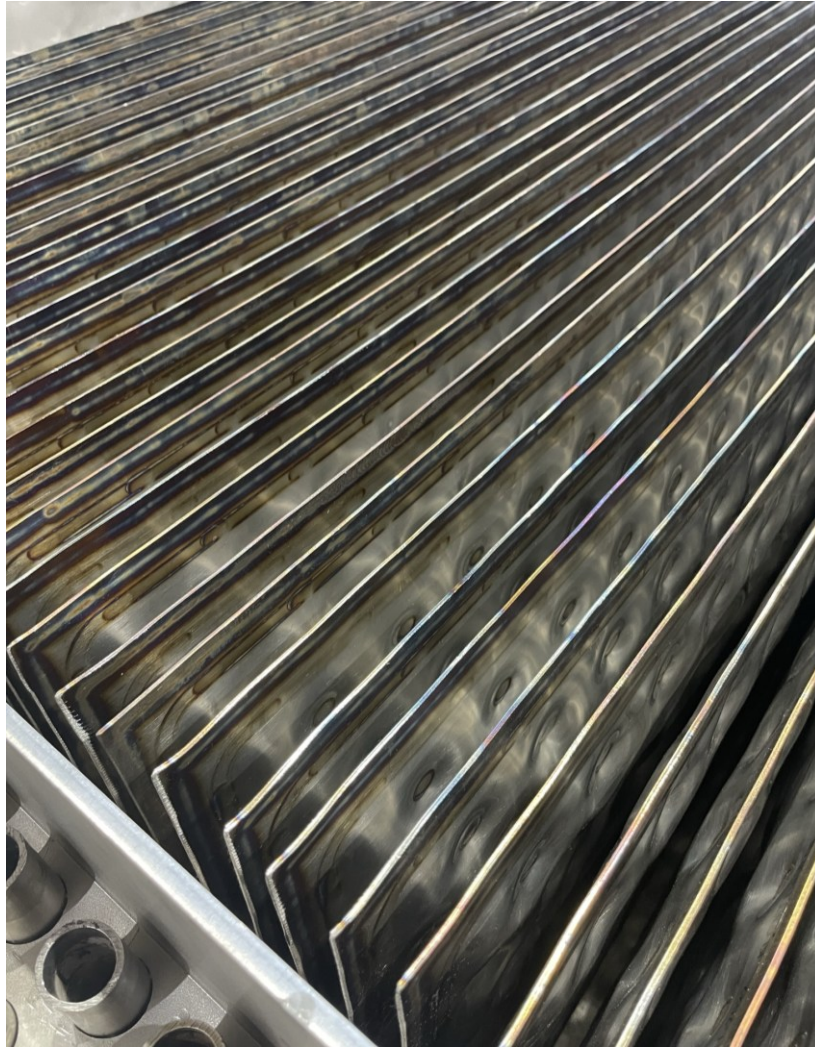
Figure 5.9: A close up to the densely stacked 904L plates, before cleaning and passivation.
