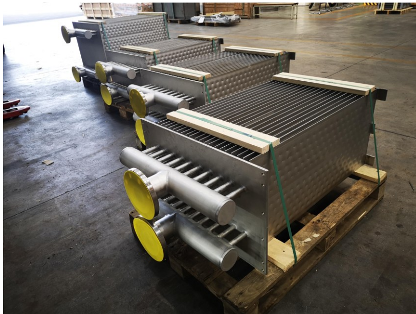
Figure 5.6: First iteration of the packed bed sand cooling PPHE, made of three identical and redundant cartridges, plus a double cartridge for heavy duty operation in the back.
