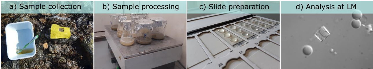
Figure 4. 1. Main steps of the treatment of diatom samples, see text for details. a) Collection of samples by brushing a known area of substratum with a 9 cm 2 template; b) oxidation of organic matter and dissolution of carbonates in the samples, on the heating plate; c) drops of diluted samples drying on the cover glasses during permanent slide preparation; d) digital microphotography at the light microscope (magnification 100x), showing three microspheres and a diatom frustule ( Odonthidium mesodon (Ehrenberg) Kützing, 1844), in girdle view.
