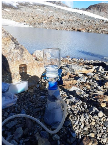
Figure 2. 6. Filtration of water samples in situ for the determination of the concentration of suspended solids in the water column.
