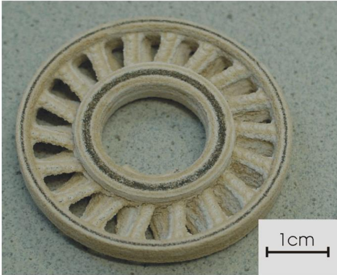
Figure 34: A model of a turbine wheel fabricated with selective laser curing and subsequent pyrolysis [160].
