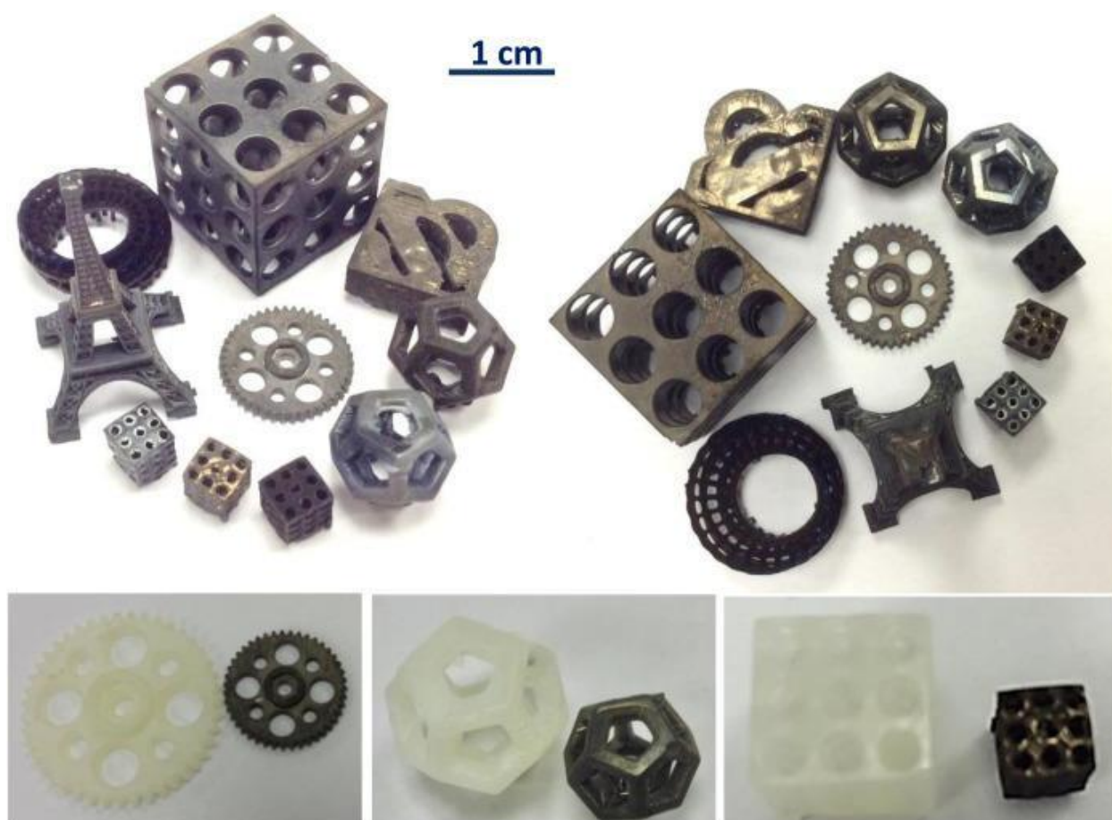
Figure 20: Ceramic parts produced from the SMP-877/BDDA mixture with stereolithography [148].
