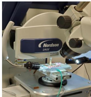
Fig. 7.10: Pull test on triplet keeping it on the carrier.
