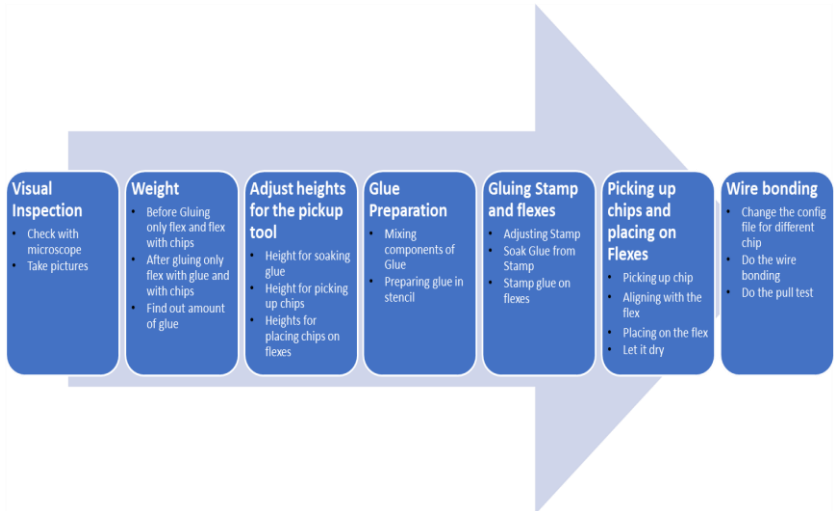
Fig. 7.5: Different steps of the triplet assembly process.
