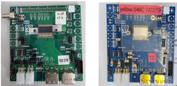
Fig. 6.9: Left is a full Single-chip card with a 3D sensor of geometry 50 \times 50 \mu\text{m}^2 1E attached with RD53A ROC and right is an SCC with a bare module, i.e ROC without sensor attached.
