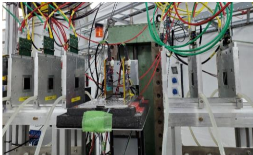
Fig. 6.23: Experimental setup in DESY with DUT in the middle of six MIMOSA EUDET telescope planes.
