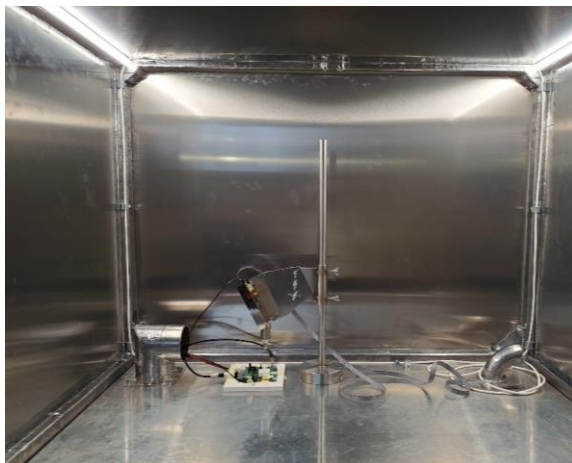
Fig. 7.17: Mini-X2 x-ray gun inside shielding box showing a source scan setup for a single-chip card.
