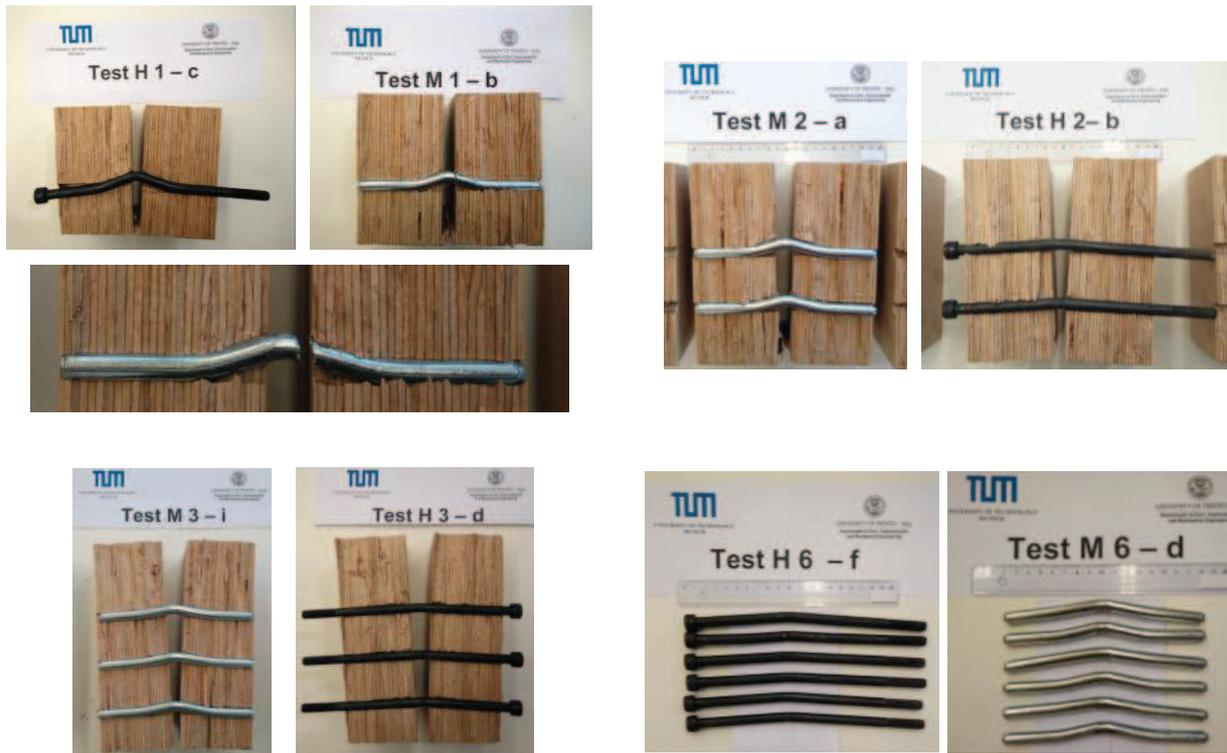
**Figure 6: Typical failure modes of each joint configuration**
