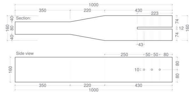
Figure 4: Joint design of the three-dowels specimen (mm).
