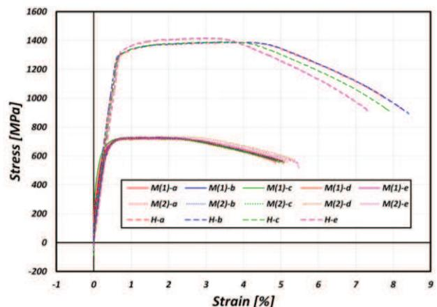
Figure 2: Tensile test stress-strain curves
