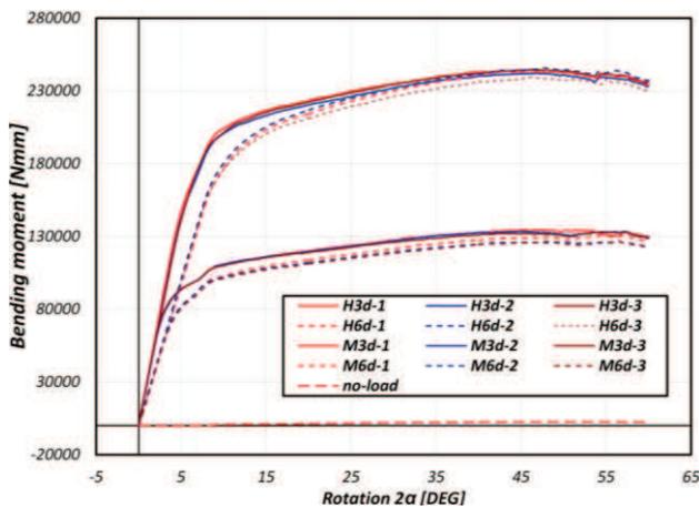
Figure 3: Bending test moment-rotation curves
