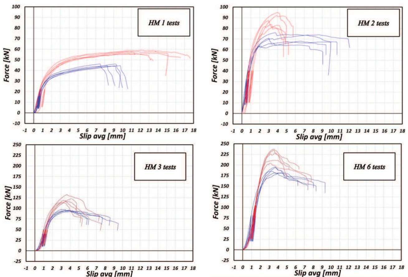
Figure 5: Load-slip curves of M-series joints (blue lines) and of H-series joints (red lines).
