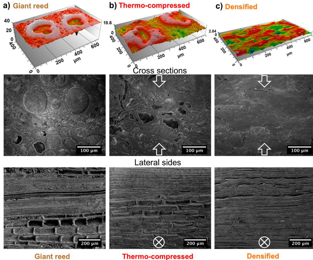
**Figure 1.** The first row of images shows the cross-section morphologies of (a) R, (b) TC, (c) D samples obtained by profilometry analysis. The second and third rows show SEM images of the cross sections and the lateral sides of (a) R, (b) TC, (c) D. White arrows in SEM images show the direction of applied pressure in the thermo-compression treatment.
