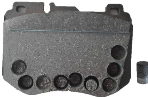
Fig. 4.1. Extraction of the pins from brake pads.
