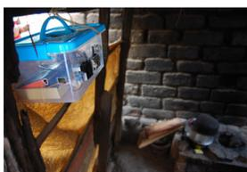
To monitor the exposition to domestic pollution (CO and PM) of local village population we carried out a sampling in Mangula village through a set of self built Arduino based sensors.
