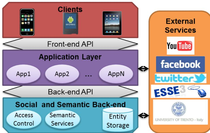
Fig. 1. Smart Campus Platform Architecture
