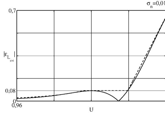
Fig. 5: Representation (solid line) of the relative error of the estimated code bin widths as a function of the transition voltage divided by the sinusoid amplitude (for null offset),  $U$ , for a noise standard deviation equal to 1% of the sinusoid amplitude. This was determined using numerical simulation. The dashed line represents the approximation given by (7).
