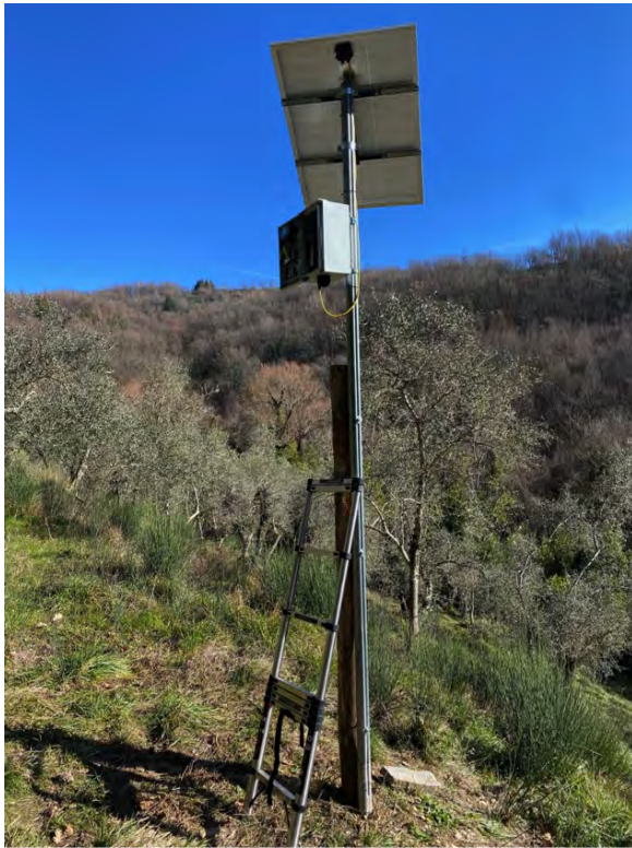
Figure 4: A SET™ (Lunilettronik.it), a station used in the Eco-Soundscape project ® for the International Institute of Ecoacoustics.
