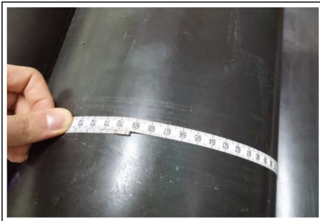
Figure 16. Pipe circumference measurement in real production (for the diameter calculation).
