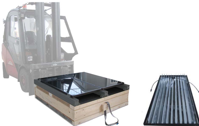
Figure 4.7: The specimen built by two enterprises belonging to the network Chi-Quadrato. The picture on the left shows the modular specimen; The other picture shows one of the two PV modules which has eleven fins attached on the back side.
