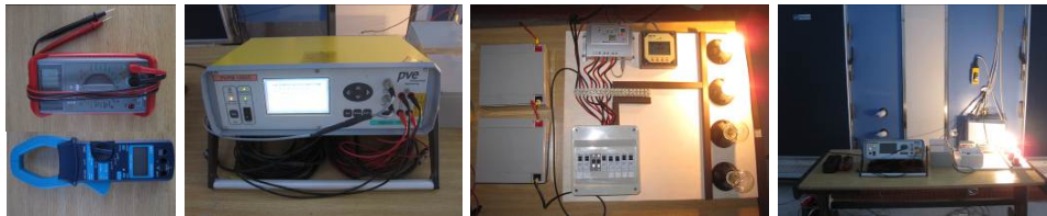
Figure 4.16: test devices used during experiments of phase 3: a current probe with a tester, a peak power measuring device with I-V-curve tracer and a stand-alone system with mppt tracer connected to the two modules. The image on the right shows the experimental setup connected to the specimen placed in the INTENT calorimeter.
