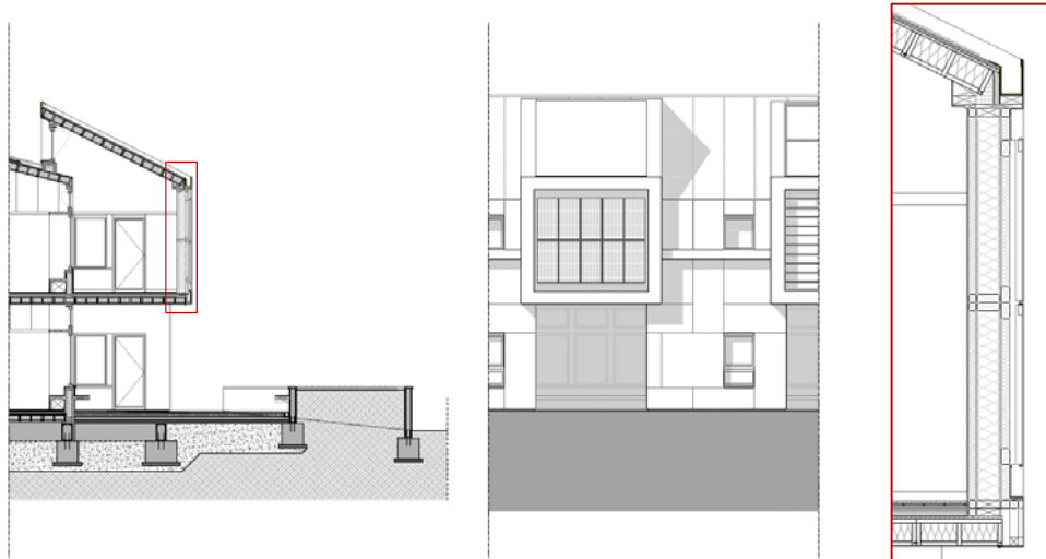
Figure 3.31: architectural drawings and details of the BiPV wall prototype integrated in the elementary school design.
