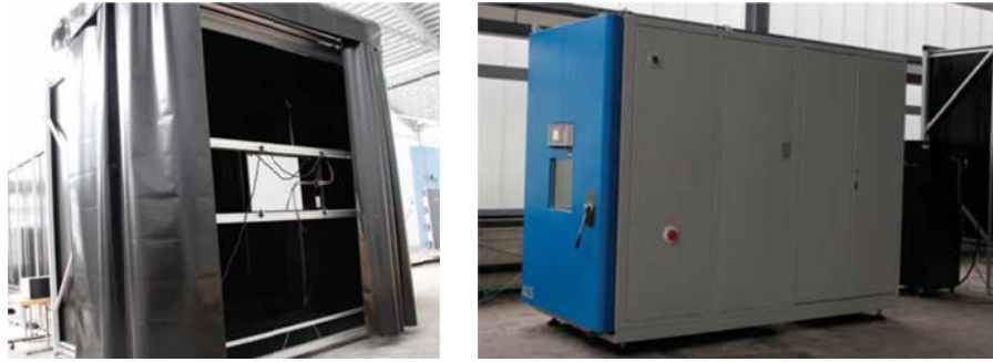
Figure 4.4: PV-SoLaRE Lab at Eurac: the sun simulator and the climatic chamber
