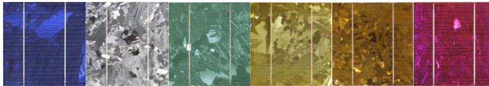
Figure 3.7: Multicrystalline silicon wafers; first the blue antireflective standard color with the best efficiency, the second is the original wafer without reflective layer, then cells with other colours that have different anti-reflective layers, © Sunways
