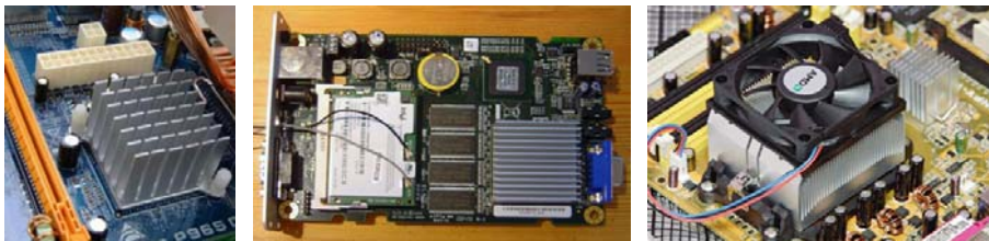
Figure 3.13: examples of CPU heat-sinks. On the right: a fan-cooled heat sink on the processor of a personal computer with a smaller heat sink cooling another integrated circuit of the motherboard
