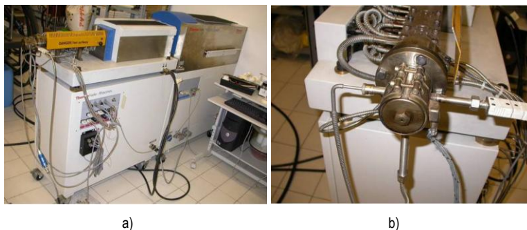
Figure 3.5. Photographs of (a) twin screw extruder Thermo Haake PTW16, (b) head of the extruder.
