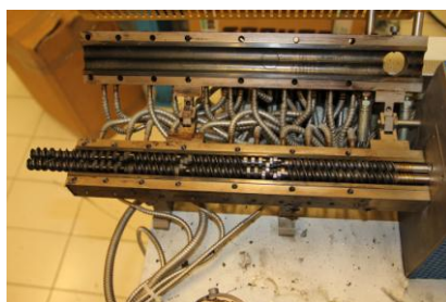
Figure 3.6. Photographs of (a) twin screw extruder Thermo Haake PTW16 view inside.
