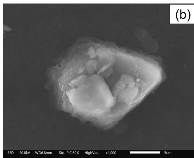
Fig. 1. SEM-SE of a single hexagonal LDH particle (a) and an example of an LDH particle cluster (b). Both images refer to pristine LDH particles without the SB addition.
