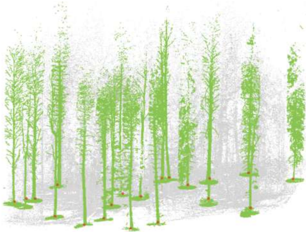
Fig. 8. Point cloud segments (green points) of each tree in a pine-dominant forest plot are delineated by considering all points in the TLS data, which are at a horizontal distance of 3b_r from the detected stem-basal center (red dot) in TLS data. The section of point cloud not belonging to the considered trees is shown in gray.
