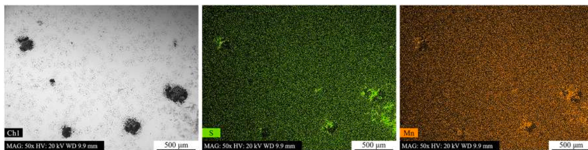
Fig. 9. Backscattered electrons SEM micrograph and EDXS S and Mn elemental mapping of the AISI 430 F* sample's bulk in the as-rolled condition after potentiodynamic polarization in 3.5 wt% NaCl solution.
