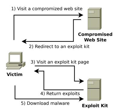
Figure 6.11: Scheme of drive-by-download attack
