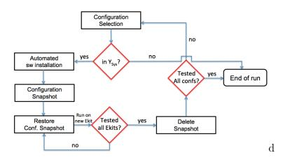
Figure 6.13: Flowchart of an experimet run. This flowchart describes a full experiment run for each system in Table 6.8. Configurations are generated in chronological order, therefore if the first control on  $Y_{Sys}$  fails, every other successive configuration would as well and the experiment ends. Snapshots enable us to re-use an identical installation of a configuration multiple times.
