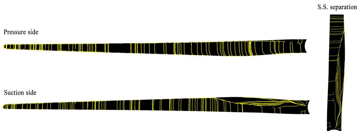
Figure 2: Blade pressure and suction side velocity streamlines - OpenFOAM (BR-CFD).
