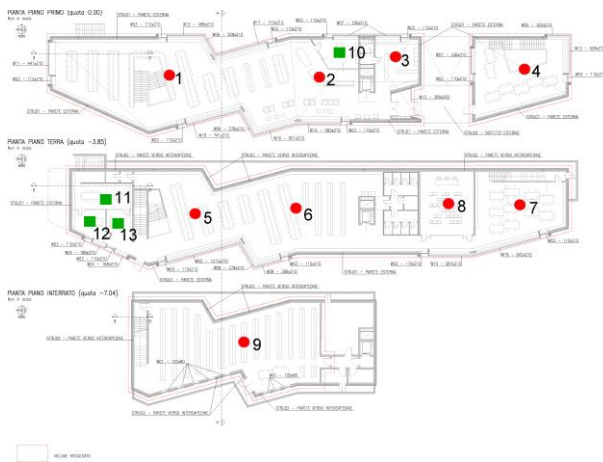
Fig. 2 – Sensor locations with their identification numbers
