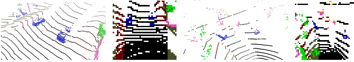
Figure 6.3: LiDAR point clouds and their corresponding BEV views: SemanticKITTI ( left ) and nuScenes ( right ). After projection, BEV images are geometrically more similar.
