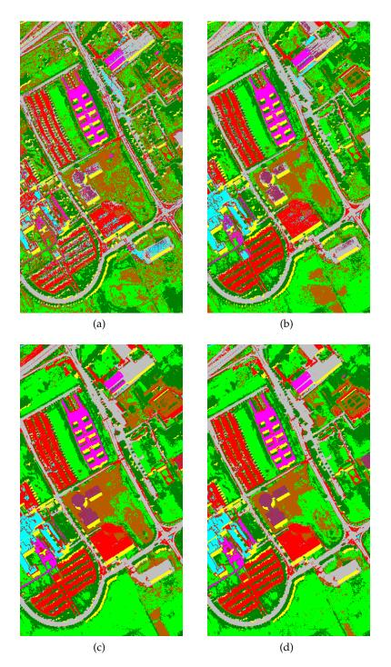
Figure 5.6: University data set. Classification maps obtained by: (a) the PCs, (b) the EMP, (c) the EAP<sub>a</sub>, and (d) the EMAP.
