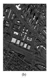
Figure 3.2: Panchromatic images. (a) IRS-1C image of the city of Athens, Greece ( $800\times800$  pixels, 5.8 m geometrical resolution, spectral range 0.5-0.75  $\mu$ m; (b) IKONOS image of the city of Reykjavik, Iceland ( $975\times639$  pixels, 1m geometrical resolution, spectral range 0.53-0.93  $\mu$ m.
