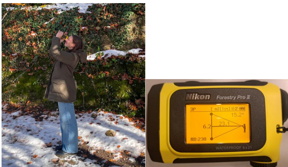
Figure 5. A student measuring tree height with a hypsometer in Mesiano Park
