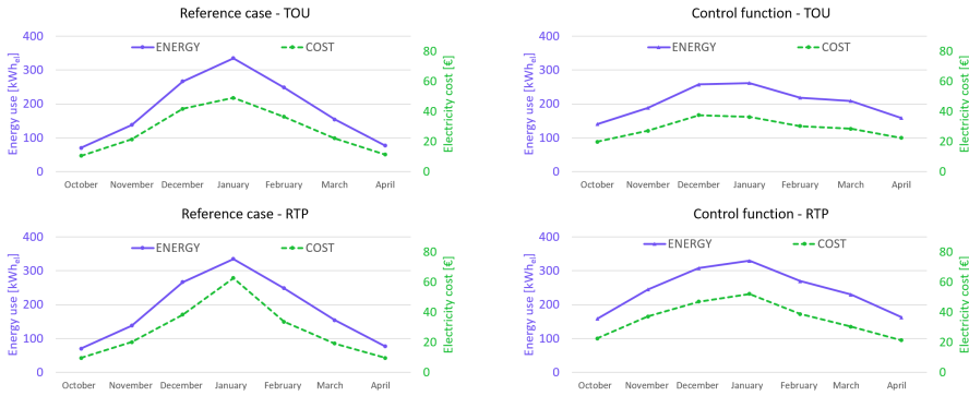
Figure 5.6: Monthly electrical energy use and relative cost for the reference case and for the case in which the control function is applied for both the time of use (TOU) pricing and the real-time pricing (RTP).
