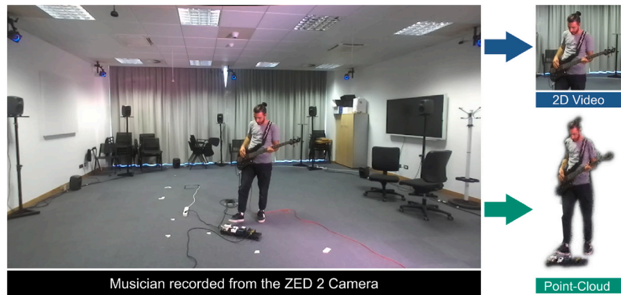
Fig. 2. The result of the Video Data acquisition: (1) the video stream of the bass player recorded on the ZED 2 camera (.svo) is rendered in Unity as a video frame and cropped (for 2D condition); (2) is rendered as a point-cloud through a shader.
