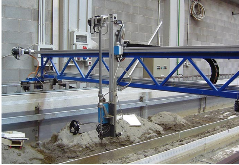
Figure 4.3: The high precision automated carriage with the monitoring equipment.
