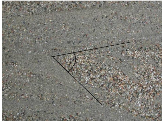
Figure 3.18: The central, wedge shaped deposit of coarse particles.
