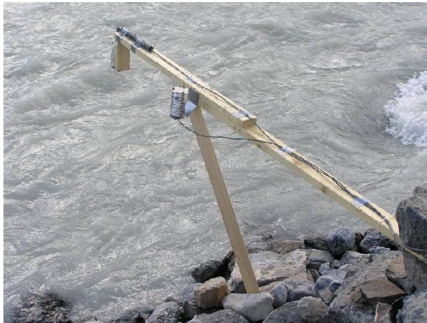
Figure 5.20: The UDG station used for free surface level measurements.
