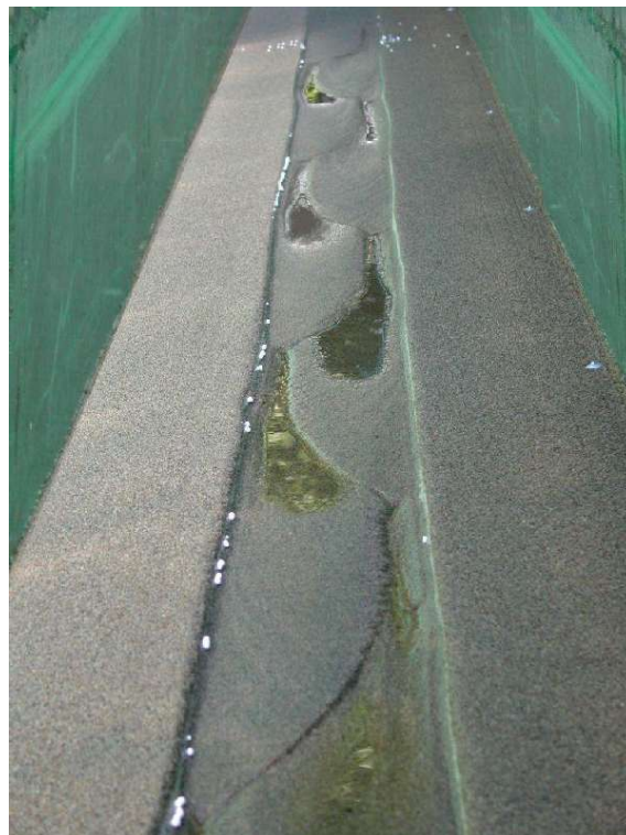
Figure 3.5: Formation of alternate bars in the early stage of channel development.
