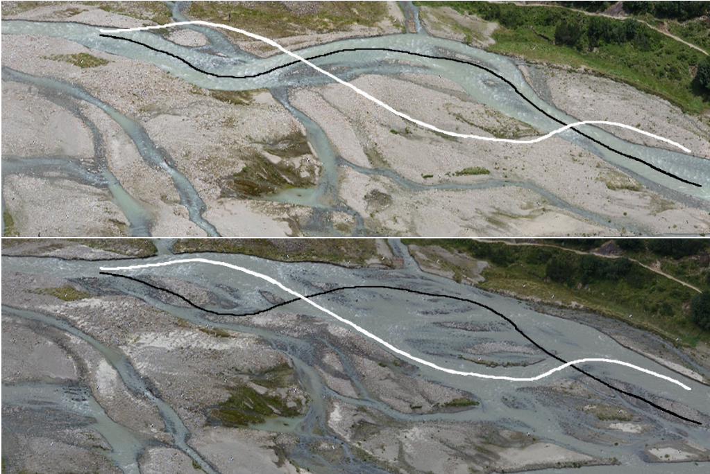
Figure 6.10: Images of the central regions of the surveyed reach in the Ridanna Creek before and after the event of July 28 th , 2003. Lines indicate the displacement of the main channel. Flow is from left to right.
