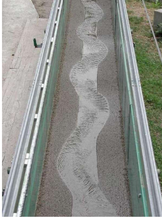
Figure 3.2: A step of the evolution of the channel: a slow meandering channel displaying regular width variations.
