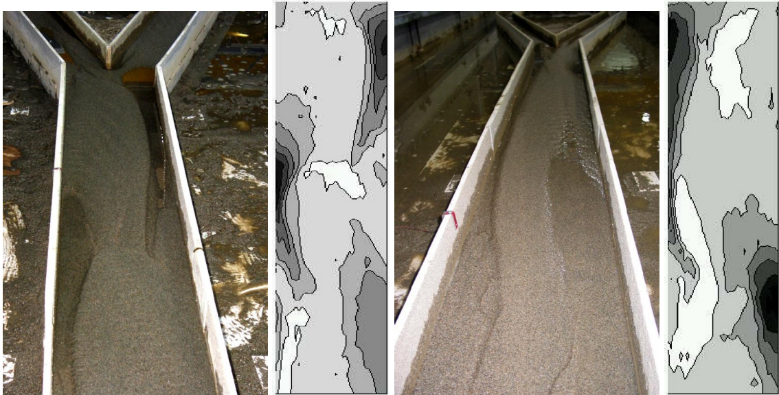
Figure 4.12: Pictures and bed topography maps of the upstream channel. Initially free migrating bars (a) and steady longer bars caused by the bifurcation (b).
