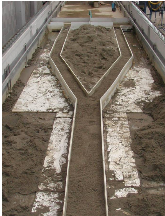
Figure 4.4: Upstream view of the 'Y' shaped configuration.
