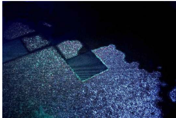
Fig. 4. Discontinuity wavefronts (some rectilinear, other curvilinear) forming during the (out-of-plane) dynamics of a periodic material (used as a toy, the so-called ‘pinscreen’, invented by W. Fleming), which works on the boundary of ellipticity loss (photo taken at the Exploratorium, San Francisco).
