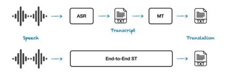
Figure 2.8: ST cascade (top) and direct (bottom) architectures.<sup>54</sup>
