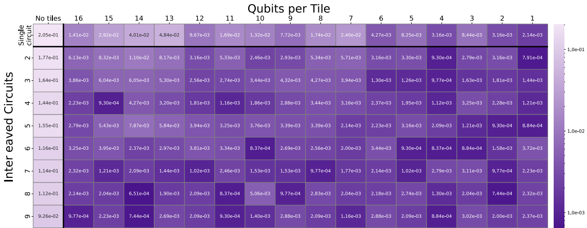
Figure 5.9: Average logical error rate of a distance-7 rotated surface code with respect to the number of interleaved independent surface codes (rows) and the number of qubits enclosed in each phonon barrier (columns) with a constant barrier permeability b_p = 0.1 , averaged over the total duration of identical radiation-induced faults.
