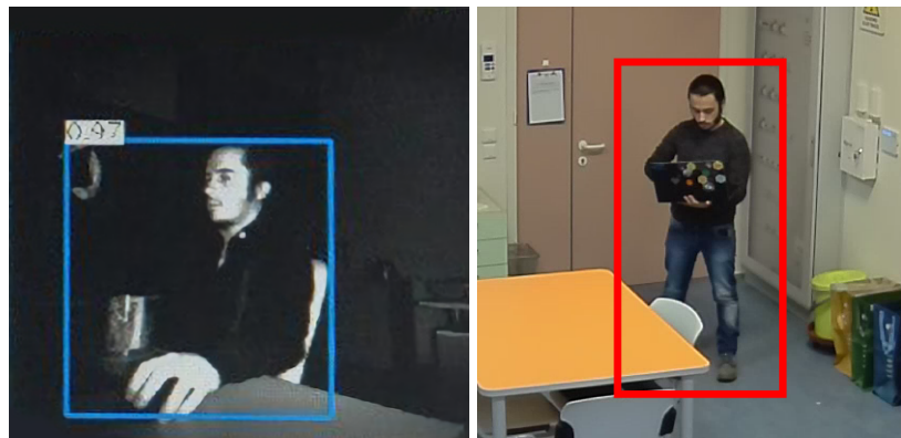
Figure 4.20: People identification through IR (infrared) sensors (left) and tracking-by-detection (right).
