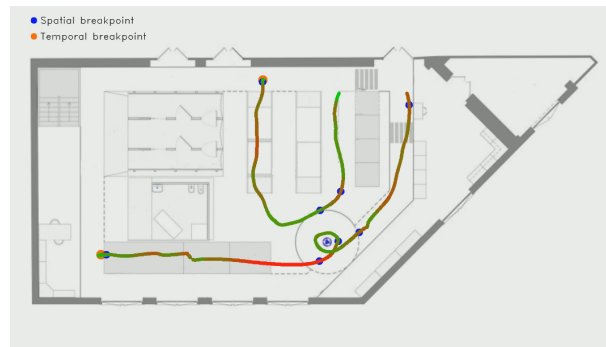
Figure 4.8: Trajectory performed by a test user projected on the gym map showing: speed changes, spatial breakpoints and temporal breakpoints.
