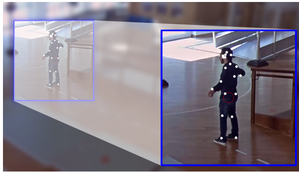
Figure 2.4: 2D pose estimation for bounding box extraction
