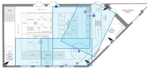
Figure 4.4: Layout of the AUSILIA gym. The environment is currently covered by four IP cameras, necessary to monitor the wheelchair path. The approximate coverage of the cameras is highlighted in light blue.
