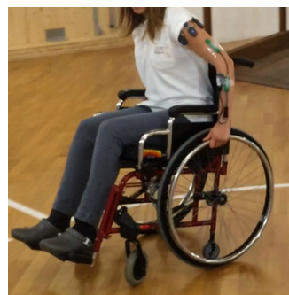
Figure 4.2: Image of a user testing all the described equipment: EMG sensors, electrogoniometer, and wheelchair.
