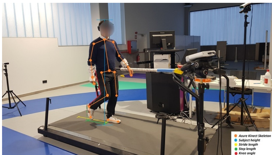
Fig. 4.7 Set up acquisition with the test subject wearing HoloLens 2 to emulate the movement of the expert user in exoskeleton walking. The colours highlight the height of the subject and some spatiotemporal parameters used for gait assessment.
