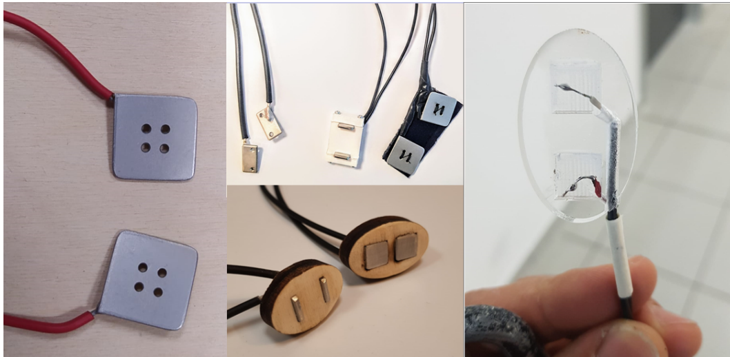
Fig. 3.2 Testing of different geometries and electrode arrangements to maximise the signal-to-noise ratio
