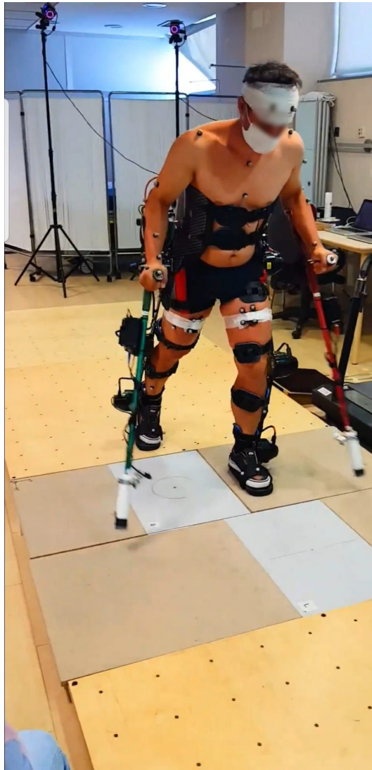
Fig. 2.2 Test of the Bullet project during exoskeleton-assisted walking with sensorised crutches and pressure matrices
