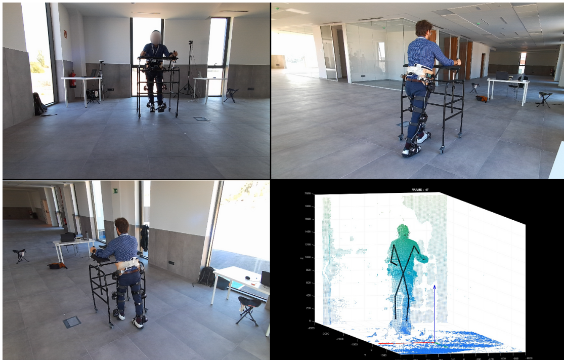
Fig. 1.5 multi-perspective view of walking with exoskeleton and walker without the treadmill returned by azure Kinect multicamera system: a) view camera 1, b) view camera 2, c) view camera 3, d) virtual reconstruction of the 3D point cloud with Azure Kinect skeleton (in black) in overlay
