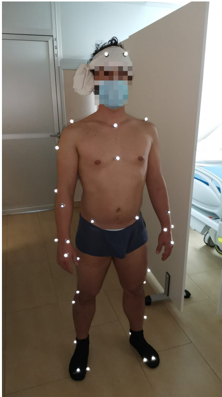
(a) Plug-in Gait marker placement of the reflective markers on a human subject for the Vicon marker-based acquisition system
