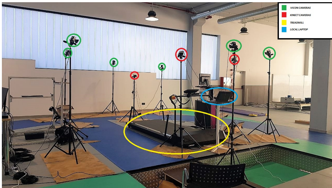
Fig. 4.2 Set up consists of six Vicon cameras, three Azure Kinect cameras, a treadmill and an AsusTUF Gaming Fx504 series laptop
