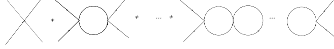
FIGURE A.1: T-matrix as infinite sum of loop corrections to the tree diagram.
