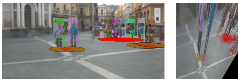
Figure 7. Algorithm output (the red circles denote the pedestrians whose d < d_{min} )
