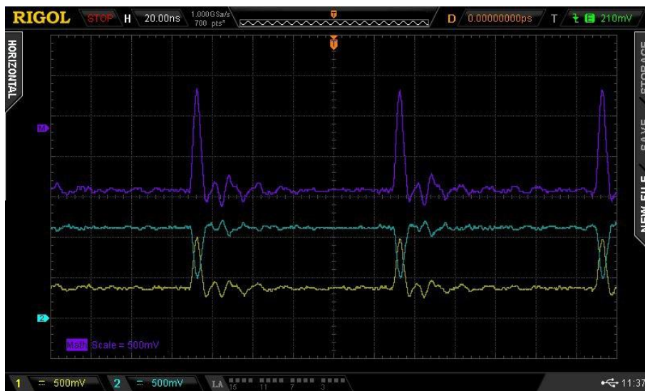
Figure 9.12: Output signal from the ABACUS board (first version). The cyan and yellow signals are measured on the CML output pins. The purple signal represents the difference between the two CML outputs, obtained with the integrated oscilloscope math functions.
