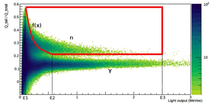
Figure 3: 2D-PSD of a  $^{252}\text{Cf}$  source, with the neutron contoured region (red line). Using the Ej-2763”x5”, the RedPitaya digitizer and the PMT model H6559.
