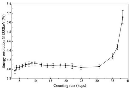
Figure 2: Energy resolution as a function of the counting rate for the CLLB detector.
