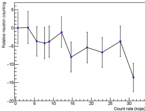
Figure 6: The relative neutron counting as a function of the total counting rate.
