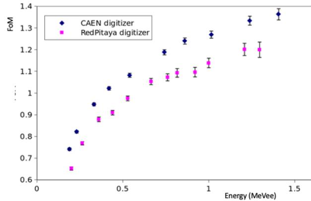
Figure 7: The FoM vs Energy for the plastic scintillator EJ276.
