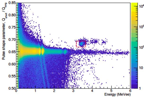
Figure 5: PSP parameter vs light output for the CCLB detector in a 15kHz gamma rate.
