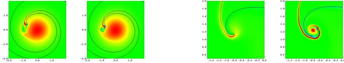
(a) Influence of Reynolds for r_\rho = 1 and We = 10^3 . Zoomed view of the vorticity field and interface at time t = 15 . Re = 10^3 (left) and 10^4 (right).
