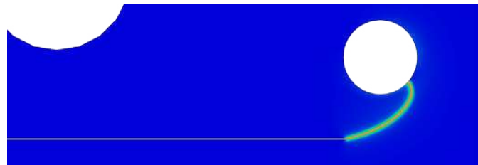
Figure 3: Phase field simulations showing the path of fatigue crack growth in a CT specimen with a hole in the vicinity of the initial crack tip subjected to cyclic tensile loading.
