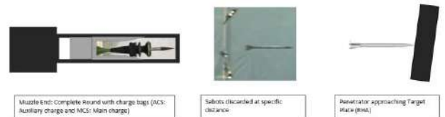
Fig 3. Experimental setup for long kinetic energy rods against RHA
