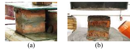
Figure 3. Compressive test: (a) specimens, (b) failure due to uniform compressive load.
