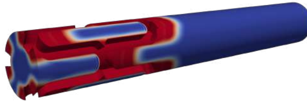
Figure 3: Drug elution in a cross-section of a Xience V stent. The figure shows a downstream clip of the stent.
