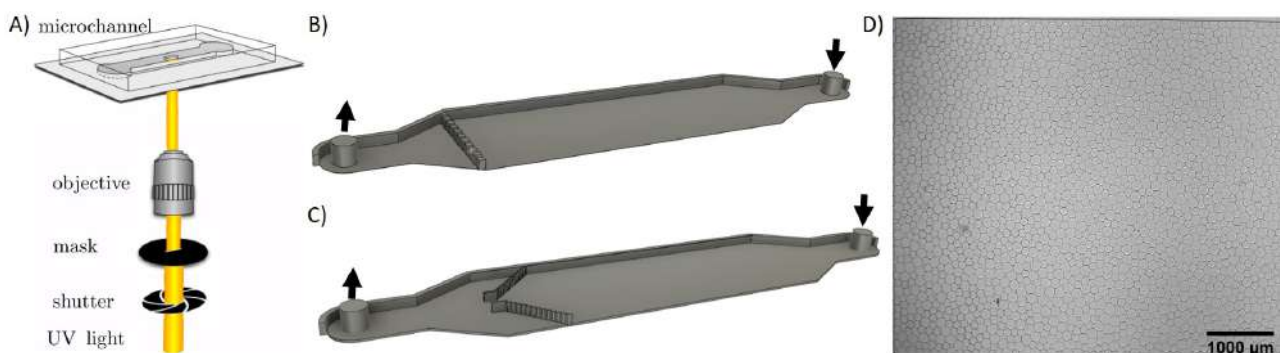
Figure 1: A) Schematic representation of the hydrogel particle fabrication (Adapted from Bechert et al. 2019 [2]). B) Example of a channel that can be used for compressional experiments. C) Example of a 2D hopper in a microfluidic channel. D) Typical packing of bidisperse particles.
