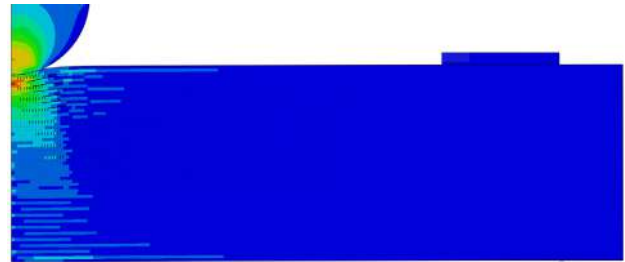
Figure 4: Example of the axisymmetric 2D numerical model simulating a 55J small-mass impact on a 20mm thick specimen.
