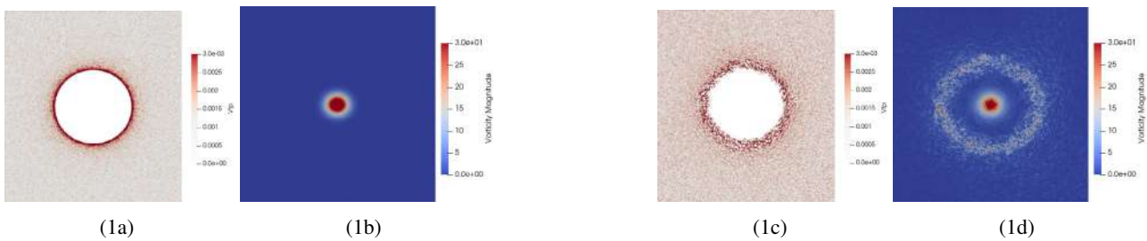
Figure 1: Particle volume fraction and vorticity magnitude at t^* \approx 1 : (a,b): one-way coupling; (c,d): two-way coupling.
