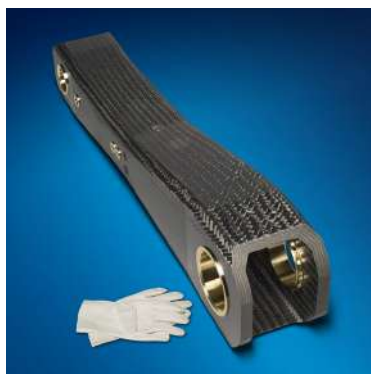
Figure 1: Demonstrator of a NH90 main landing gear trailing arm.
