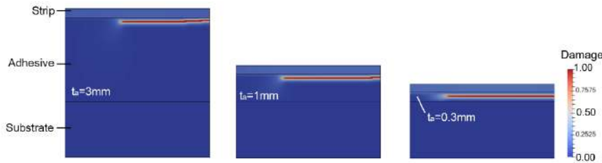
Figure 2. Details of the crack path evolution from the models with different thicknesses of the adhesive.
