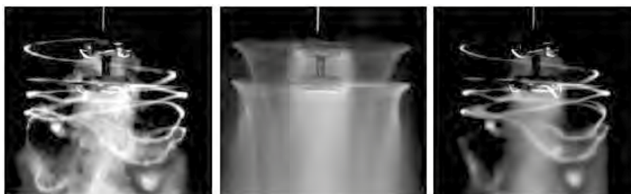
Figure 2: An instantaneous image, time averaged image and phase averaged image (25 samples) at H/R = 0.41 and 6 rps.
