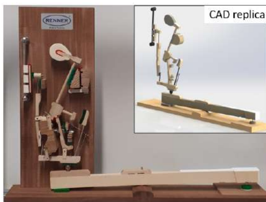
Figure 1: Upright piano action demonstrator and its equivalent CAD replica.
