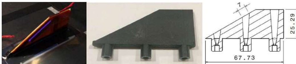
Figure 3. Actuators on vortex generators: plasma (left) and air jets (center and right).
