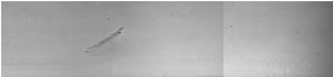
Figure 1: Experimental realisation of growing turbulent stripe at Re=750 (flow from left to right).
