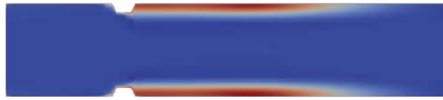
Figure 2: Drug elution in a cross-section of a one-strut simplified stent configuration.
