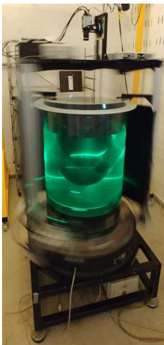
Figure 1: Details of the experimental setup. Left : Picture of the experiment after the spin-up is completed. The tank is 1.6 m high, 1 m in diameter and rotates at 75 rpm. Right : height and \beta as a function of the cylindrical radius.
