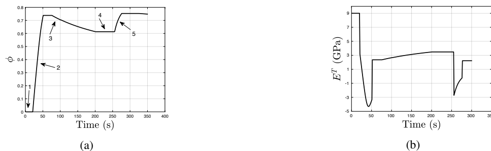
Figure 3: (a) Variation of effective damage with time (b) Variation of algorithmic tangent modulus with time
