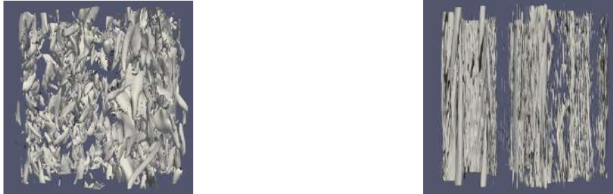
Figure 1: Helicity isosurfaces without and with magnetic field in unstably stratified periodic box turbulence.
