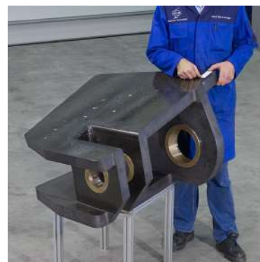
Figure 2: Gear rib of the Affordable Low Cost Aircraft Structures (ALCAS) airliner wing [1].
