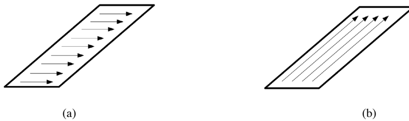
Figure 3 : Two raster strategies with which the block (shown in Figure 2) can be produced (a) Raster X (b) Raster Y
