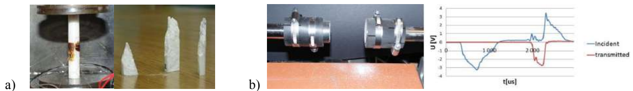
Figure 2. Failure modes of CMC for: a) splitting in quasi-static loading (MTS) and 2) crushing during impact loading with SHPB.
