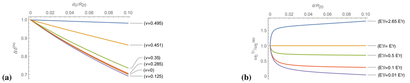
Figure 2: (a) Ratio of the damping constants \delta/\delta^{inc} , with \delta^{inc} = \delta(K' = \infty) , for \mu_K = 0.7\mu_G and (b) undamped resonance frequency \omega_0^T/\omega_0 for different ratio between the orthoradial and radial Young moduli. Poisson coefficients are set to 0.3.
