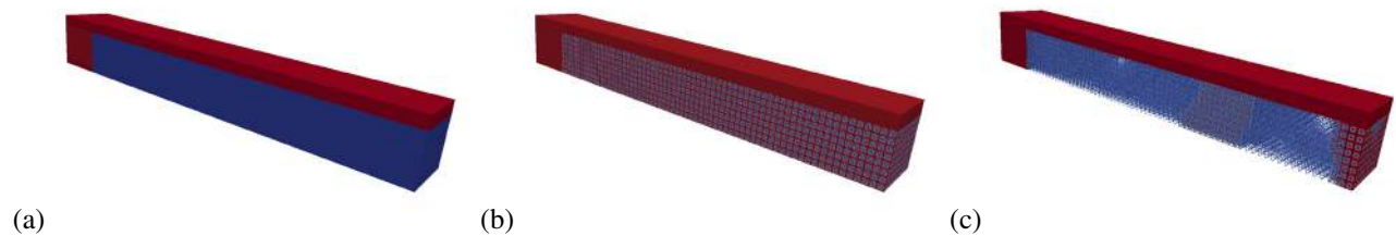
Figure 2: (a) Part (red) and support structure (blue), (b) minimal support structure with a spatially uniform density distribution, and (c) minimal support structure with a spatially varying density distribution.
