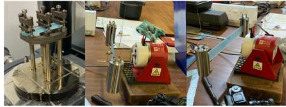
Figure 1: DMA and the vibration experiment setups
