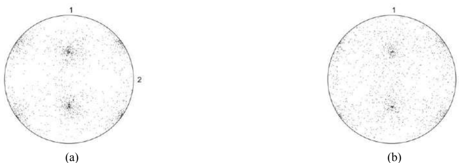
Figure 1: \{111\} pole figures for Goss texture corresponding to a series of Gaussian distributions of increasing scatter width : (a) \omega=25^\circ and (b) \omega=35^\circ .
