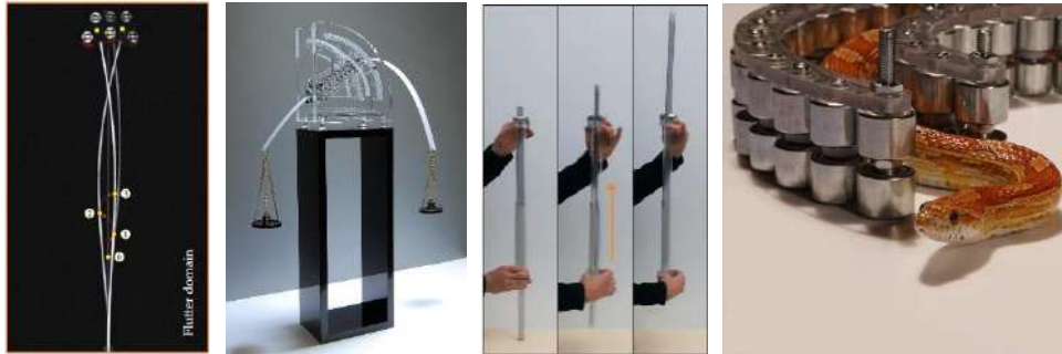
Fig. 2 From left to right, models for: Flutter instability; The elastica arm scale; The torsional gun; Snake locomotion
