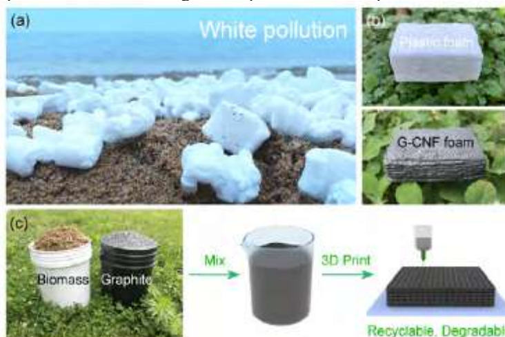
Figure 1. Photos and schematics demonstrating the replacement of the white pollution using bagasse and graphite that are recyclable, degradable and printable. (a) The white foam pollution. (b) Digital images of plastic foam and G-CNF foam. (c) Schematic of the recyclability and degradability of the printed G-CNF aerogel made from the plants and graphite mine in nature.
