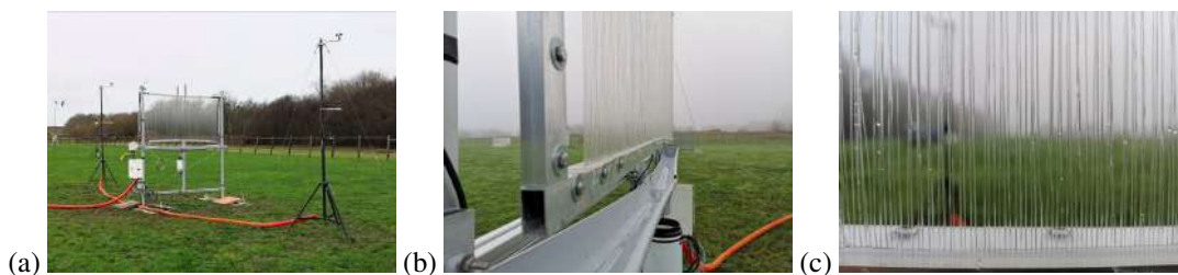
Figure 1: Set-up for fog collection measurement with vertical fibers on the SIRTa. (a) Complete set-up : The fog collector, 2m long, 1m high, on a supporting structure ; One rain gauge of 0.1mm resolution ; Four wind sensors : two on the West side, two on the East side; Three force sensors: two on each upper corners of the frame, one on the bottom side, in the center. (b) Water flowing in the gutter to the rain gauge at the bottom of the collector. (c) Zoom on the pairs of nylon fibers stitched to PVC plates.
