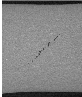
Figure 1. X-ray absorption image of an aluminium alloy specimen indicating the localization of damage into an interior microcrack.
