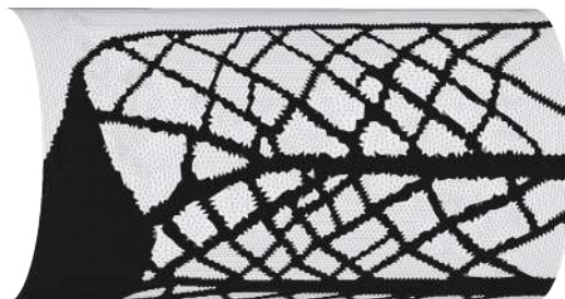
Figure 1: Geometrically nonlinear topology optimization based flexure design on a cylindrical surface. The design is suited for laser cutting.
