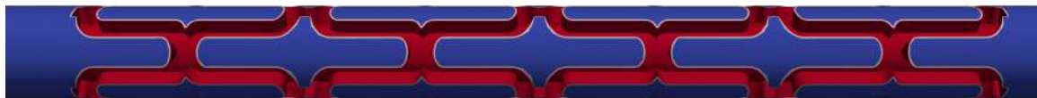
Figure 1: Crimped geometry of the Xience V stent. The stent struts are highlighted in red.
