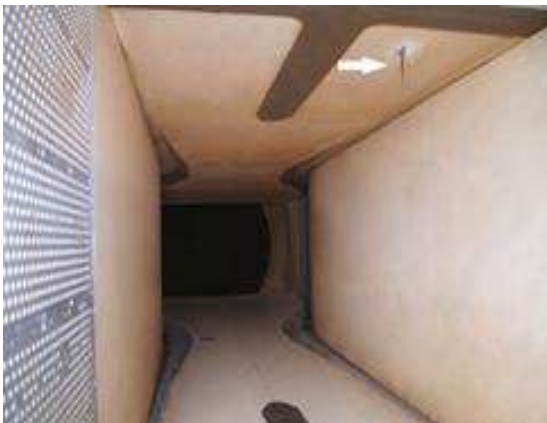
Figure 1. Wind tunnel nozzle and rake installed on its upper wall.
