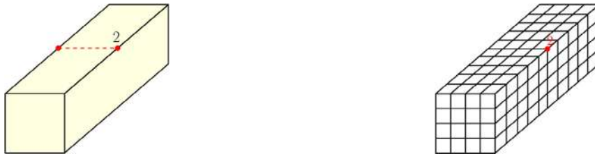
Figure 2 : Lower region of the part shown in Figure 1, discretized with hexahedral elements
