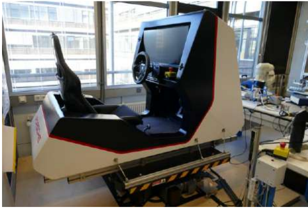
Figure 1. Setup of the presented Driver-in-the-Loop (DiL) simulator with a Porsche racing simulator, a Stewart motion platform and an Optitrack motion capture system consisting of four cameras attached to the ceiling.
