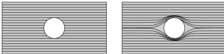
Figure 1: Comparison of two fiber orientation samples (left: uniform, unidirectional fiber orientation – classical technology, where the fibers are drilled; right: fibers bypassing a hole)
