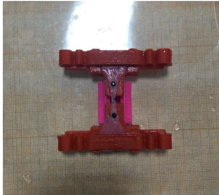
Picture 1. The specimen after the experiment. (Visible rupture can be observed at the middle)
