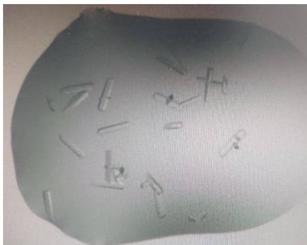
Fig 36. Crystal of PP1/PTG 81-107 grown in 0.1 M Tris pH 8, 1.6 M Lithium sulfate, 1.4 M Sodium malonate pH 6.0
