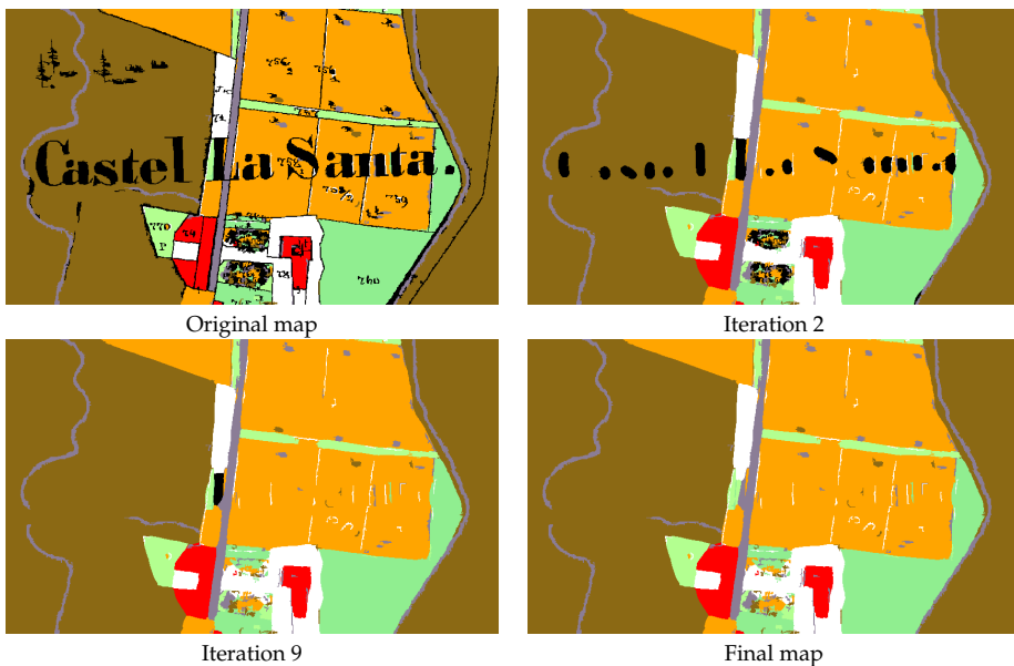
Figure 12. Text, symbol and lines removal with 23 \times 23 filter: original map, map after two and nine iterations and the final map, with all text, symbols and lines removed, after 24 iterations.
