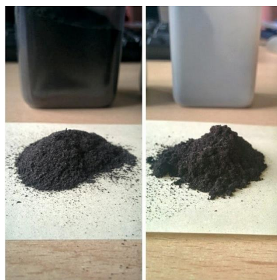
Figure 5: Char from apple pruning residues (on the left) and from wood pellets (on the right)
