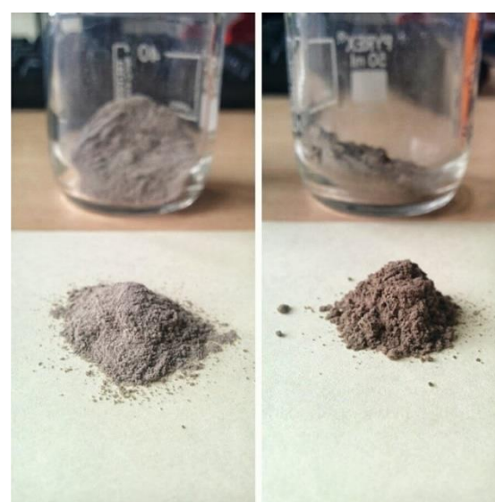
Figure 6: Ashes obtained from the apple pruning char (on the left) and from wood pellets (on the right)
