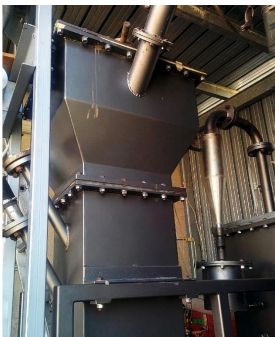
Figure 2: Main body of the reactor (on the left) and cyclone with the tank (on the right)
