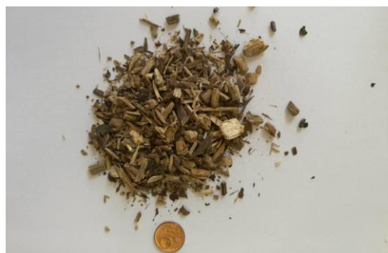
Figure 1: The residues of apple pruning that were fed to the spouted bed gasifier
