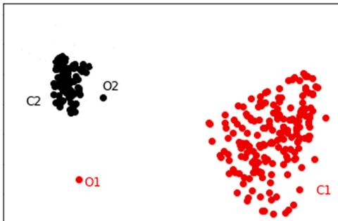
Fig. 2. A sample dataset that contains two clusters of data ( $C_1$  and  $C_2$ ) and two outlier objects ( $o_1$  and  $o_2$ ).
