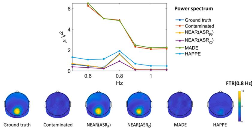
**Fig. 4.** Top panel: Power spectrum of the simulated *frequency-tagging dataset* between 0.5 and 1.1 Hz, averaged over the electrodes showing the largest FTR amplitude in the *ground truth* data (PO3, POz, PO4). Bottom panel: Topography of the FTR (defined in Section 2.3.5) at 0.8 Hz (the stimulation frequency). (For interpretation of the references to colour in this figure legend, the reader is referred to the web version of this article.)
