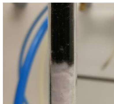
Figure 3: Char (above) and quartz wool (below) inside the quartz reactor
