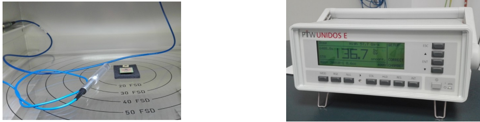
Fig. 3.3: The x-ray dose measurement system composed by a calibrated Farmer Chamber probe (left) and a PTW electrometer(right).
