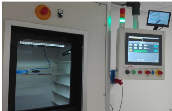
Fig. 3.2: The x-ray shielded irradiation volume. The x-ray tube is located on the top of the irradiation volume.
