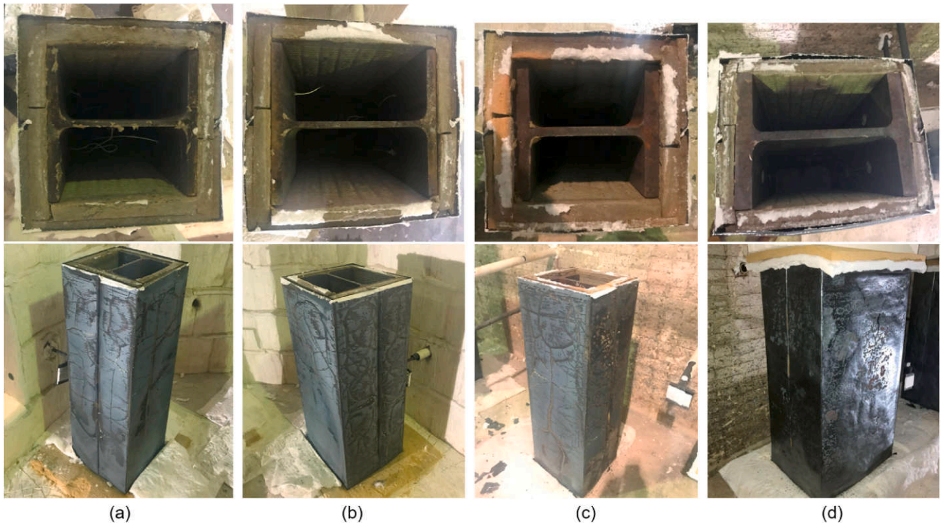
Fig. 28. Unloaded specimens after the 120 min of exposure to standard fire: a) Specimen 8; b) Specimen 9; c) Specimen 10; d) Specimen 11.
