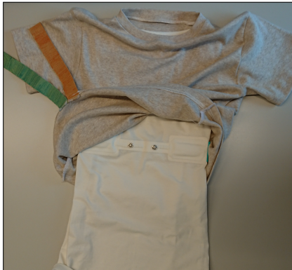
Fig. 1. Example of a prototype sensorized garment designed for children with ASD. The two metal buttons present on the white jersey allow the connection of the textile electrodes with the sensing unit (not shown).
