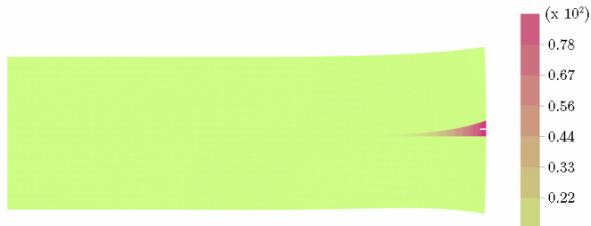
FIGURE 4.6: Post-elastic behaviour of the analytical model showing normalised average strain (average strain divided by maximum average strain in the body) upon crack nucleation for the chosen load distribution. The displacement of the configuration are scaled by a factor of 100 in order to make the deformed shape appreciable.
