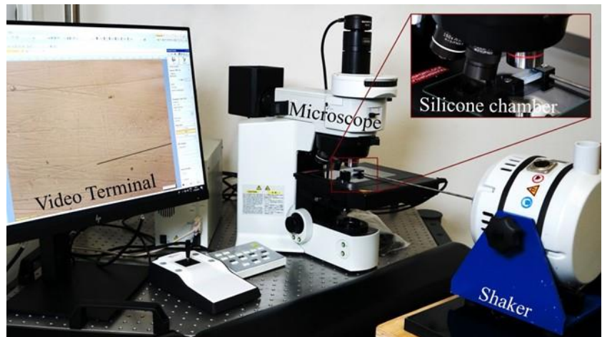
Figure 5.1 Final set-up of the experiments. The silicon chamber containing the fibre embedded in gelatin was placed under the object lens of the microscope. As highlighted
