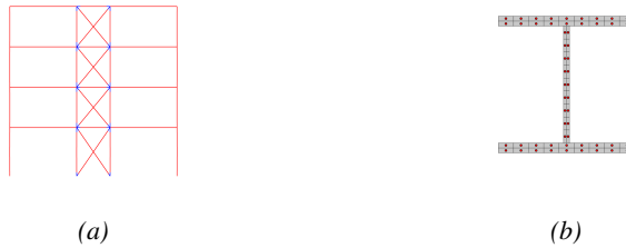
Figure 9.5: a) advanced 3D frame modelled in OpenSees: nonlinear elements in red, elastic elements in blue; b) Fiber Section.
