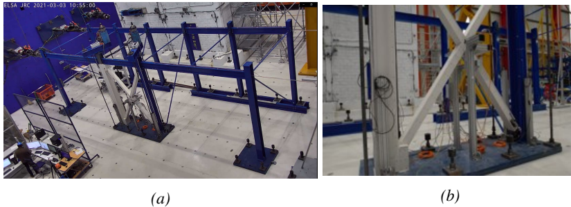
Figure 8.44: a) General view of the specimen and experimental setup at the ELSA Reaction Wall; b) detail of the brace.
