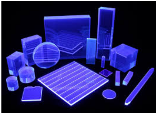
FIGURE 1.7: Plastic scintillators under UV light excitation [16].
