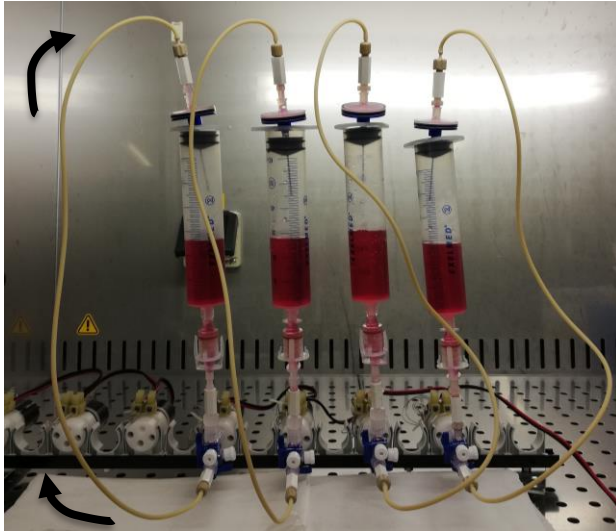
Figure 18: final set up of the homemade bioreactor, using the components reported in Fig. 17. In the image, it is possible to observe as the syringes work as medium storage to allow the recirculation of the medium (clockwise direction, black arrows) and to keep the system self-sustaining for long time.
