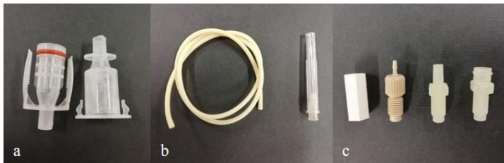
Figure 17: different components used to build up the homemade bioreactor: a) sterile chambers in which the scaffold was inserted; b) marprene tube and needle and c) various connectors.
